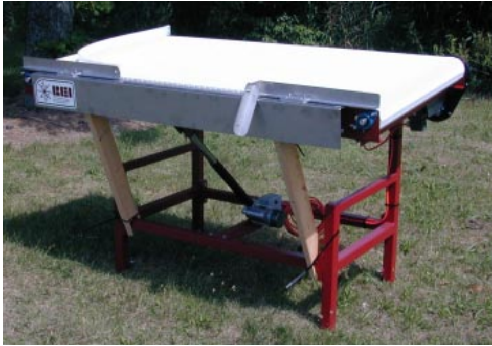
Picture shows Tilt Belt with shipping braces
